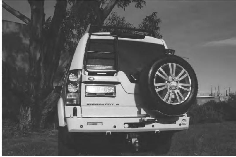
5. A padlock should be fitted to the lock tab protruding through the rear of the wheel mount. If a padlock is fitted, it must be cable tied to the main upright of the carrier to prevent it moving. Padlocks on jerry can holders, can be tied through the holes provided.
