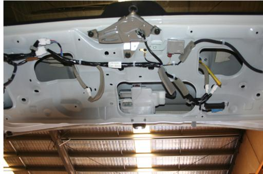
7. On the inside of the tailgate undo the four nuts securing the chrome camera/numberplate housing to access the camera.
