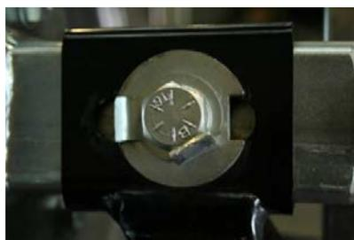
11. Please stick on 3M plastic film (provided) to the bar where the latch is situated to protect the bar finish.
