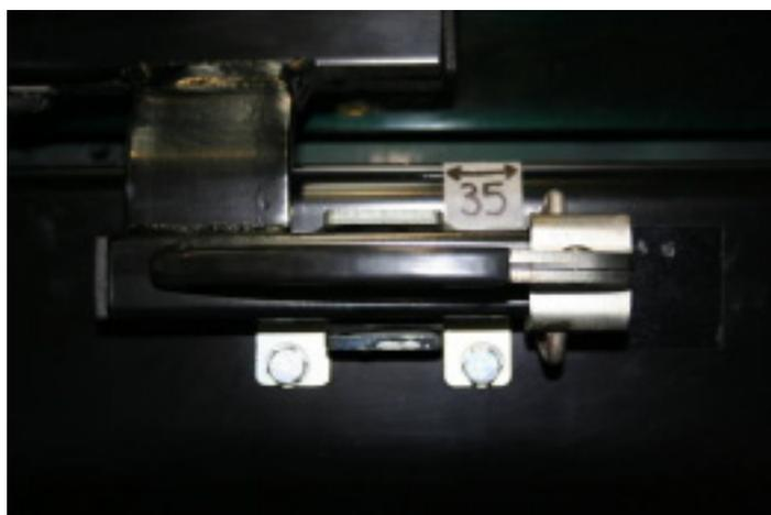
10. The hook of the lock catch can be levered in or out to give a positive tension when locking the handle closed.
