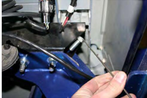
6. Fit bolt plate into chassis down through support gusset in Kaymar bar using M12 flat, spring and nut. **DO THESE BOLTS UP FIRST.**
