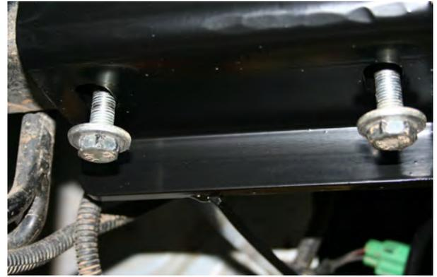
18. Check that the bar sits evenly side to side on vehicle add packers between inside of chassis and Kaymar bar to centralize. Fit eight x (four either side) M12 x 35 x 1.25 bolts, springs and flat washers to eight x captive nuts in chassis
