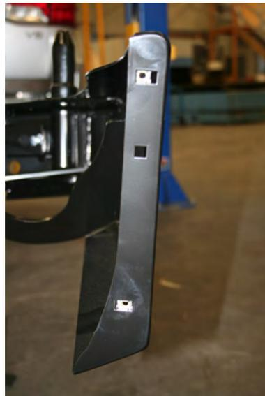
14. Slide the plate with 2 nuts welded on, into the right hand side of chassis lining up with the 2 holes in the bottom of chassis
