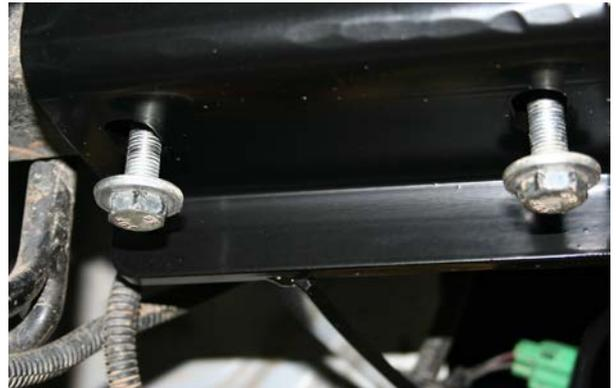
18. Slide the 3mm packer between the bottom of the chassis and the bar. Do up these bolts first then tighten the remaining bolts
