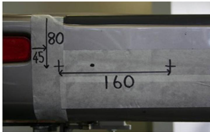
2. Mark bumper as per photo. Drill two outer holes to 6mm and hole for wiring to 10mm. About 50mm in from screw holes.
