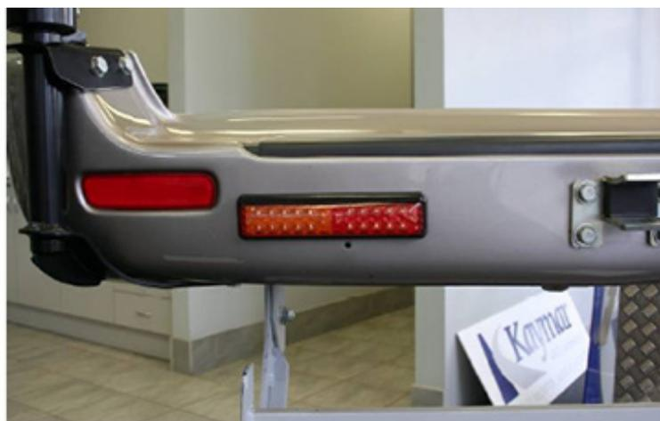
4. Feed wiring through 10mm hole. Clip LED lens back into housing.
