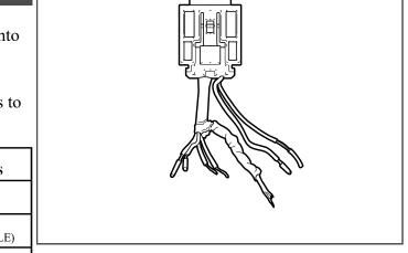
• Ensure to maintain twisted section of the 2 twisted pairs (L. Blue & Red and Blue & Green) of the 4 core wires to obtain good camera signal. Use electrical tape to wrap the twisted section.
