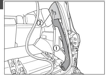
• Dislodge the Rear RHS section of the Roof by pulling it down via the white plastic clips. Do not pull directly on the trim material(1).
