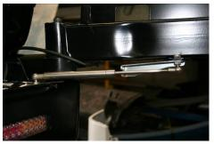
3. Using the carrier arm for leverage, compress the strut and slide the carrier arm completely on to the pivot shaft. Fit the greased top bearing, flat washer and nut. Tighten firmly (but not over tight) and fit the split pin.
