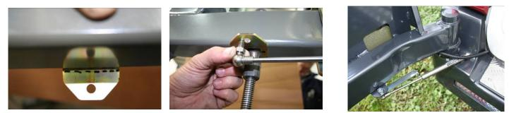
Note: With this bracket clamped into position, a measurement of 270mm should be achieved between the two hole centres.
