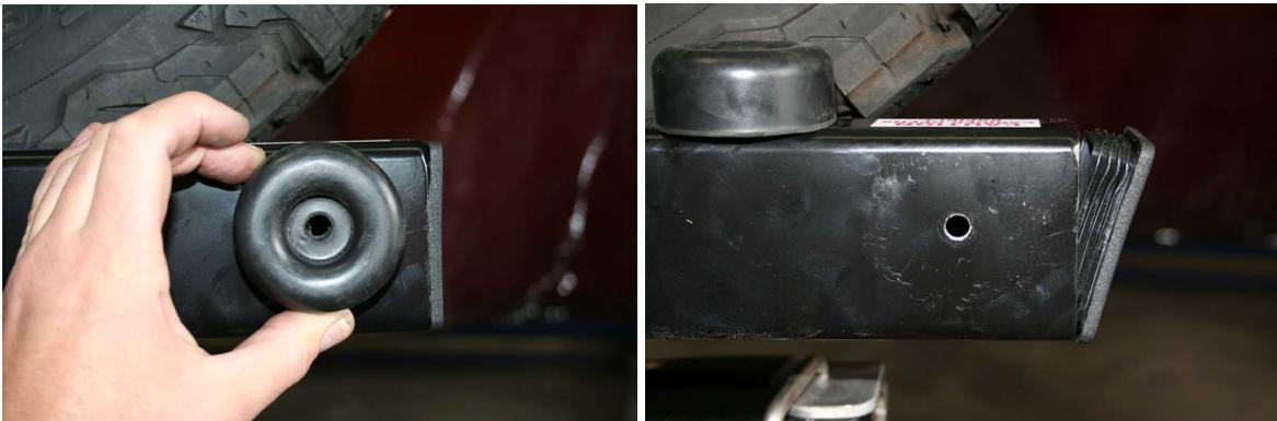
3. Remove the end cap and fit the bump stop using M10 x 1.5 x 30 bolt, spring and flat washers and wizz nut.
