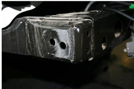
15. Fit two M12 x 50 x 1.25 bolt, flat, spring washer to either side into bottom of chassis.
