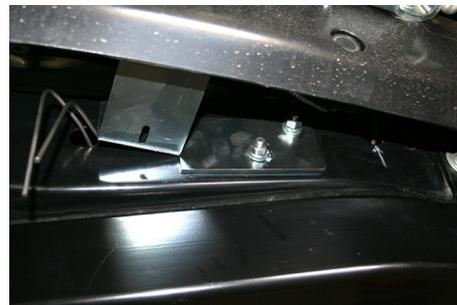
5. Fit sensor to the bracket using 3/16 screws provided.
