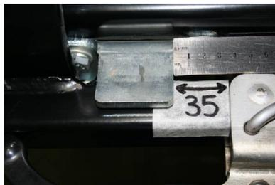
17. Move the lock catch along the handle rail until you achieve the 35mm gap as shown in above picture. With the lock catch held firmly against the vehicle with the carrier, mark the position of the bottom two holes of the lock catch.
