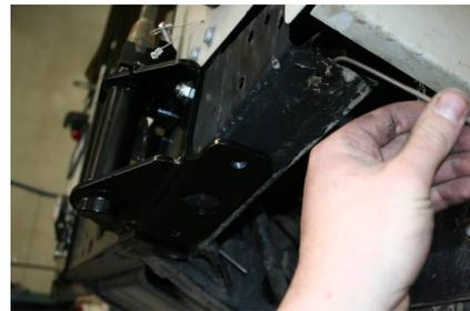
11. The second support brace needs to be drilled to ½ inch.
