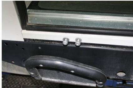
6. Some holes in chassis need to be enlarged. See photos below and drill to 11mm.
