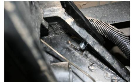
13. Fit M12 bolt through the bottom brace. Secure using M12 flat, spring and M12 nut.
