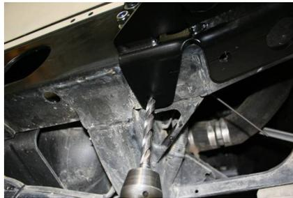
12. The top brace, must be fitted. This slides between the body and the top of the chassis. Fit 12mm bolt through the hole in chassis gusset, underneath the body. Fit two M10 bolts with washers, through the two matching holes in corner bracket. Using M10 flat, spring and M10 nyloc nuts.
