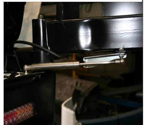
strut fits through from the underside of the tab on the carrier arm. Attach using M8 nyloc nut. Leave loose.
