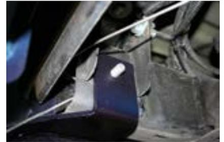
6. Fit M12 x 1.75 x 30 bolt through top of spring hanger, down through plate at end of pipe gusset. Secure using M12 flat, spring and nut. **TIGHTEN ALL BOLTS.**
