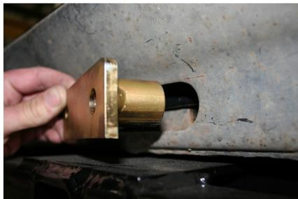
11. Fit 8mm packers between chassis and top of bar arm. Tighten these bolts first, then all other bolts.
