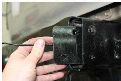
2. Slide the square plates with captive nuts and wire into the chassis rail. Make sure you have the correct one, as these are made left and right.
