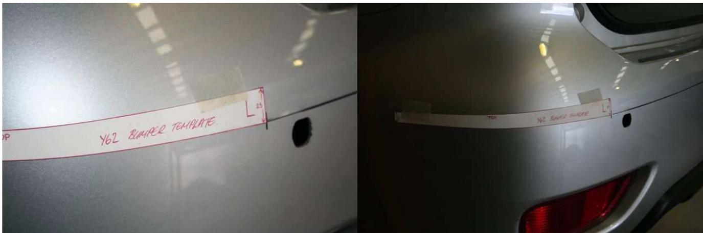
12. Measure down from where bumper meets body at wheel arch 100mm. Mark and with a ruler join line across to where template line finished.
