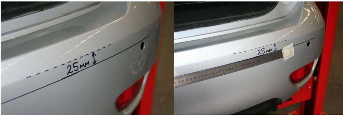
10. As seen in photo below, hold a ruler vertically against edge of bumper. Mark this position as this is where the cardboard template sits.
