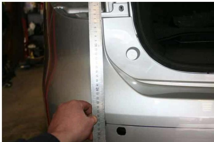
11. Position cardboard template on this mark. Making sure template is on the correct way. (TOP) is up and (L) or left is facing toward centre of vehicle. Wrap template around bumper corner following natural line in bumper. At the mark, flip the template over and mark right hand side the same way.
