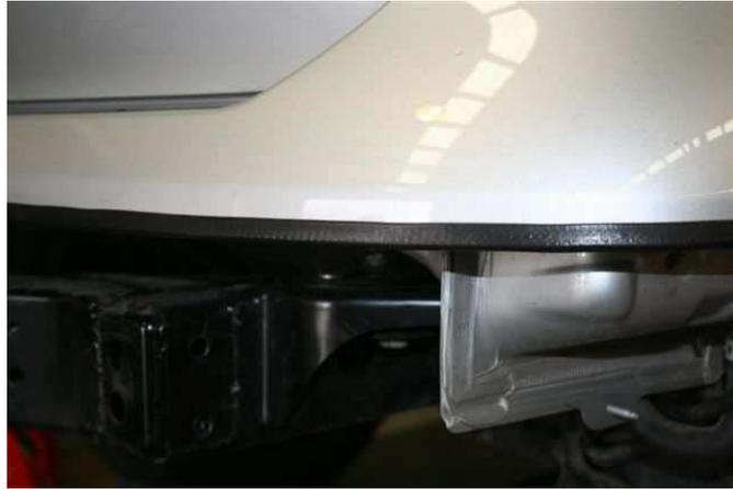
15. On either side of chassis, are two captive nuts, knock out nuts, then drill holes to 1/2".
