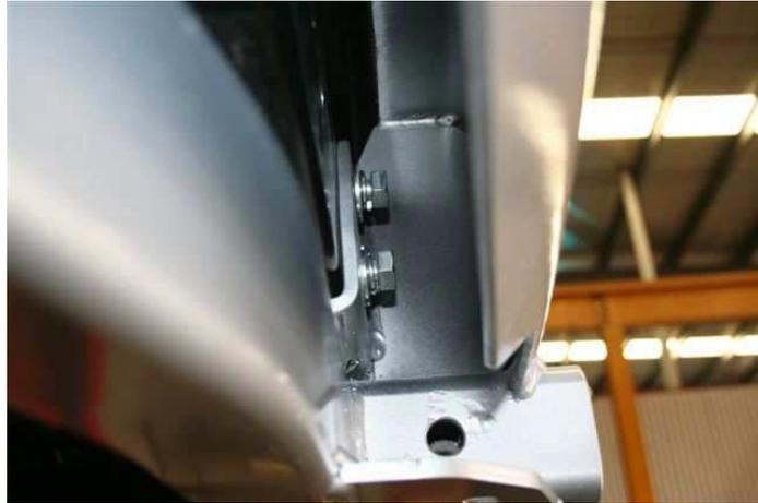
18. Fit 4 x 2 either side – bolt on wire, through rectangular hole in chassis out through holes you drilled earlier using M12 flat, spring and nut.
