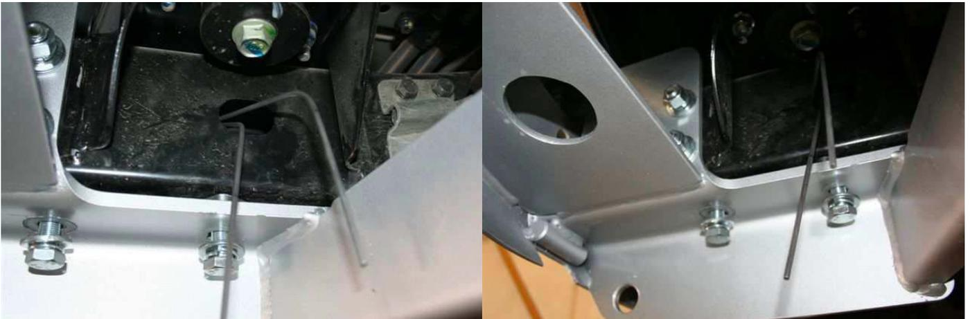
19. Tighten 6 x bolts in the bottom of chassis first. Sight along wing and bumper cut, there should be an even gap of 5-8mm. 3mm packers are supplied for any variation in body to chassis.
