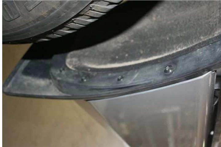
22. Mark position of where mud flap bolt to original brackets. Drill out to 8mm and attach using original hardware.
