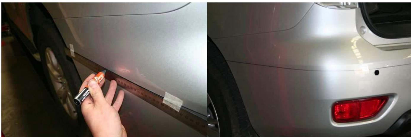
13. Check all measurements are correct. Then using a grinder with cutting disc. Cut on line. If cutting bumper while bumper is on vehicle, be careful not to cut through any vehicle wiring eg:- sensor harness.
