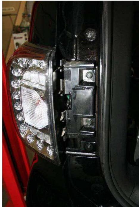
3. Gently pull tail light assembly towards outside of vehicle to release plugs. Un-plug wiring harness from behind light and put light aside.
